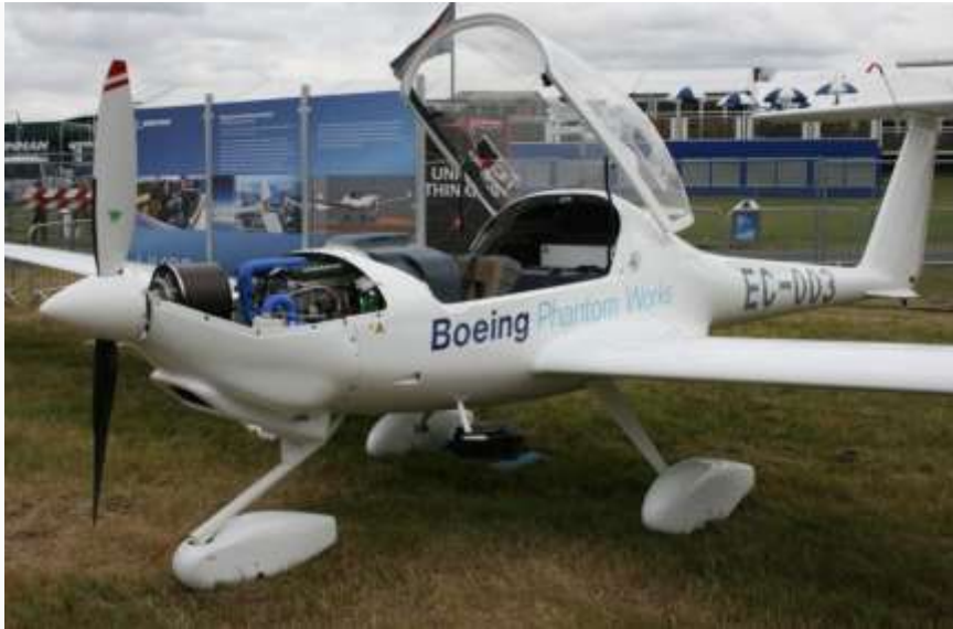
Boeing flew the first hydrogen fuel cell-powered aircraft in 2008. Photo: Adambro via Wikimedia
