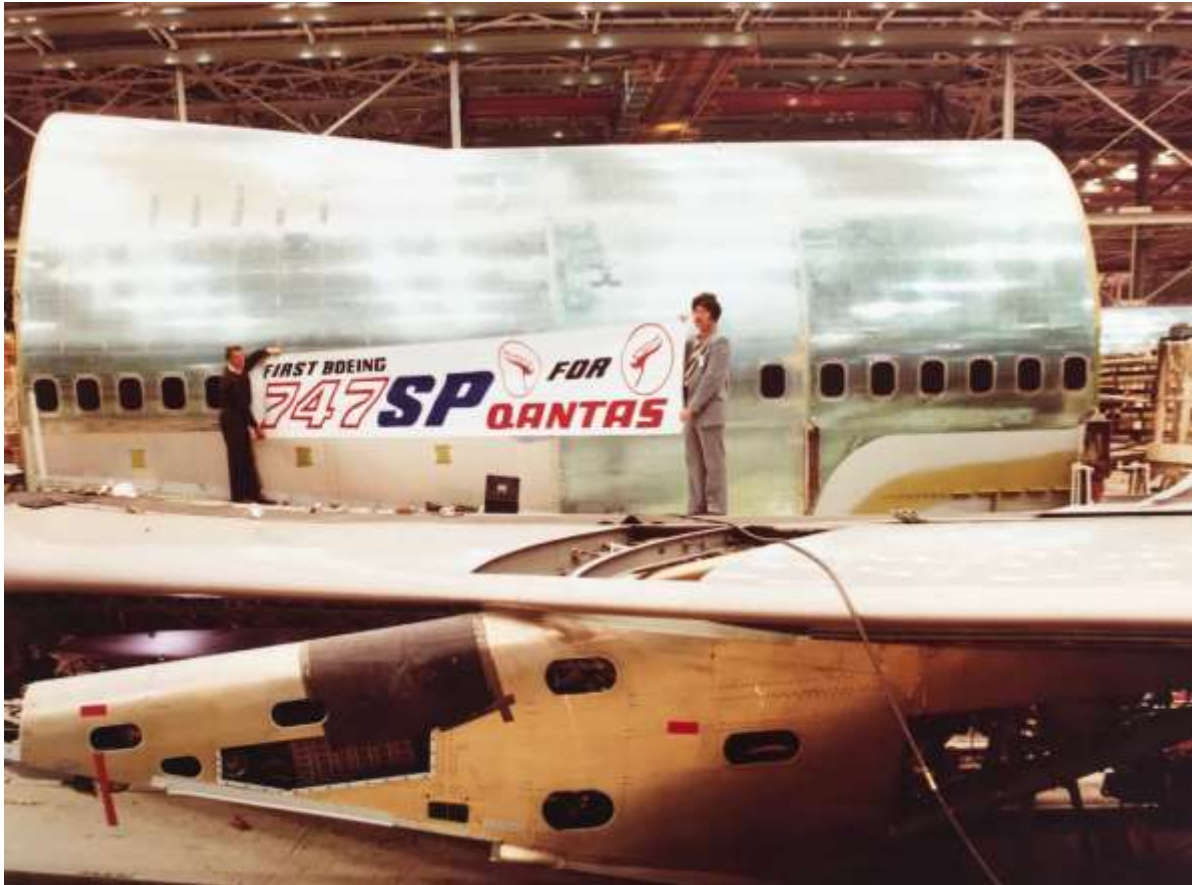
The first Qantas Boeing 747SP, VH-EAA, during production. Bill and the Qantas production inspector are on the wing.
